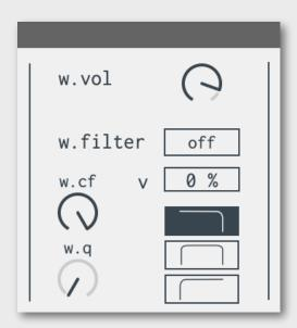
Each sound generator (waves & noise) passes through a **Sallen & Key filter** (designed by Surreal Machines, more info at the end of this user guide), with the following controls:
