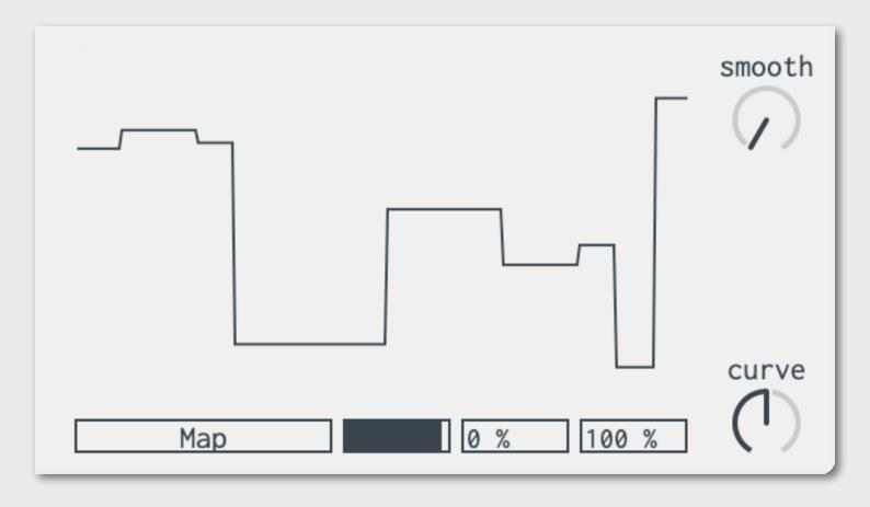
To the right of the device, you'll find a **Signal Monitor** that shows you how your sequence translates into the control signal being sent out.
