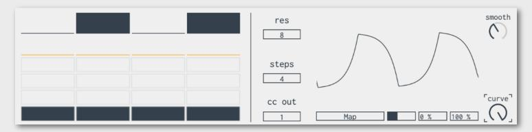
In this third example, the curve is set to an extreme **positive value** (it takes an exponentially longer time for the signal to rise up or fall down)
